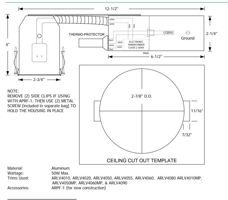
3" Clearance all around and 2" above is required when installed
