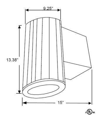
OUR OVAL WALL CYLINDERS FEATURES AN EXTRUDED ALUMINUM HOUSING WITH DIE CAST BALLAST HOUSING, INTERNAL ALUMINUM REFLECTOR, AND CLEAR TEMPERED GLASS LENSES. FIXTURE IS AVAILABLE AS A DOWN LIGHT, OR AN UP & DOWN LIGHT. FLUORESCENT UNITS INCLUDE OUR 42N1 ELECTRONIC BALLAST AND 42W LAMP(S). FINISHED IN OUR NINE-STAGE POWDERCOAT PROCESS FOR ADDED PROTECTION IN MOST HARSH ENVIRONMENTS. UNIQUE WALL MOUNTING BRACKET FOR QUICK & EASY INSTALLATION. HINGED BALLAST COMPARTMENT WITH SAFETY CABLE.
